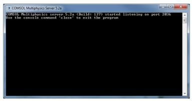
When the COMSOL Multiphysics Server starts, it listens for a COMSOL Multiphysics Client connection on the port listed in the command window. In the example above it is port 2036.
