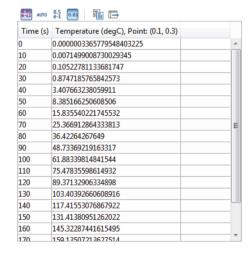
The source of the results table data is one of the child nodes to **Derived Values** or **Tables** under **Results**. In the figure below, a **Table** node is used as the source (by selecting this option in the tree and then clicking **Use as Source**.)
