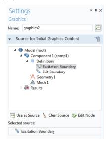
When a graphics object is linked directly to a selection in this way, the graphics object displays the geometry and the user can interact with it by clicking on the boundaries. The boundaries will then be added (or removed) to the corresponding selection.
