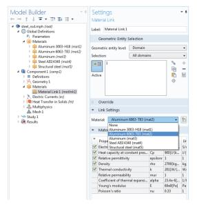
Each material is indexed with a string: mat1, mat2, ..., mat5. An event listens for changes to the value of the global variable alloy, where the value is controlled by a combo box. When the value is changed, the method listed below is run.
