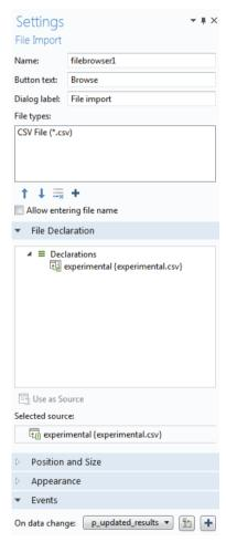
In this application, the **File types** table specifies that only CSV files are allowed. The **Settings** window for the **File** declaration is shown in the figure below.
