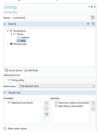
Note that the **Alloy** combo box uses both the **Aluminum Alloys** and the **Steel Alloys** choice lists. The choice list for **Aluminum Alloys** is shown in the figure below.
