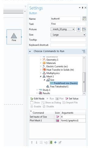
In the above example, a **Set Value** command is used to set the value of the **Predefined mesh size** (hauto) property. The property **Predefined mesh size** (hauto) corresponds to the following settings in the **Size** node shown earlier:
