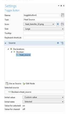
Enabled corresponds to the Boolean variable heat\_source being equal to true, which in turn corresponds to the toggle button being selected. Disabled corresponds to the Boolean variable heat\_source being equal to false, which in turn corresponds to the toggle button being deselected.
