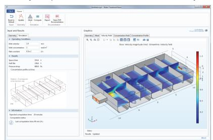
The exemplified system is a chlorination basin in a water treatment process.
