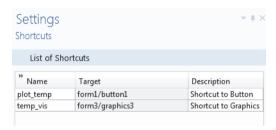
The shortcuts can be referenced in other form objects or in code in the Method editor. The example below shows a shortcut, temp\_vis, used as an input argument to a temperature plot.
