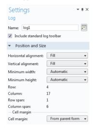
The figure below shows a part of an application user interface containing a log window.
