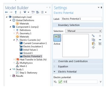
The figure below shows the **Settings** window for an input field. The list of possible sources for this field now contains the **Electric potential**.
