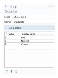
To learn which values are used by the **Element size** list in the model, use **Record a New Method** and change the value from **Normal** to **Fine**, then to **Coarse**, and then back to **Normal**. Click **Stop Recording** and read the values in the autogenerated code. The **Element size** property name is hauto and the values for **Fine**, **Normal**, and **Coarse** are 4, 5, and 6, respectively, as implied by the automatically generated code shown in the lines below.
