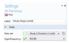
In the **Editor Tools** window, the **Eigenfrequency** parameter is visible as **Loop Level**. To create a combo box, right-click **Loop Level** and select **Input**.
