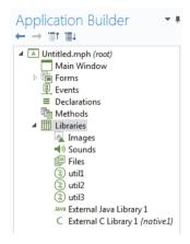
The embedded files can, for example, be referenced in form objects or in methods by using the syntax embedded://file1, embedded://file2, and so on. For example, to reference the image file compute.png, use the syntax embedded://compute.png.
