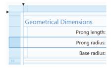
Similarly, to select a column, click the cell at the top. This cell cannot contain any form objects. The figure below shows the third column highlighted. In this case, the **Column Settings** menu is enabled in the ribbon tab.
