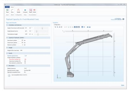
In this application, a rigid-body analysis of a crane is performed in order to find the payload capacity for the specified orientation and extension of the crane. This application also provides the usage of hydraulic cylinders and highlights the limiting cylinder. The capacity of the hydraulic cylinders can be modified in order to improve the payload capacity and the usage of the cylinders.
