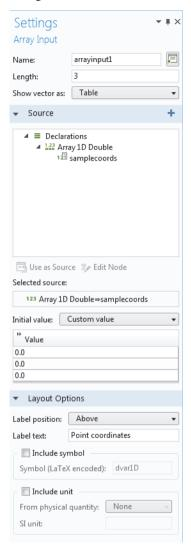
The Array Input form object uses a Source named samplecoords, which is a ID Array of type Double. This array is created prior to the creation of the Array Input object by declaring an Array ID Double with the following Settings.
