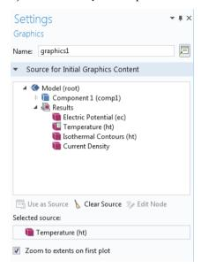
In addition to **Results** plot nodes, you can also use **Selection**, **Geometry**, and **Mesh** nodes as the **Selected source**.
