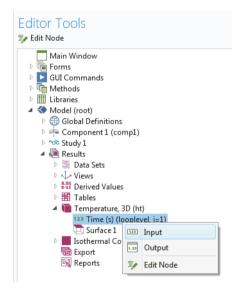
By selecting **Input**, you can create a combo box using it as **Source**, as shown in the figure below.
