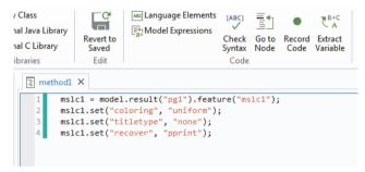
The code starting with the prefix feature has been replaced with the variable mslc1. When you click the **Extract Variable** button, an **Extract Variable** dialog box opens where you can enter a suitable variable name in the **Name** field.
