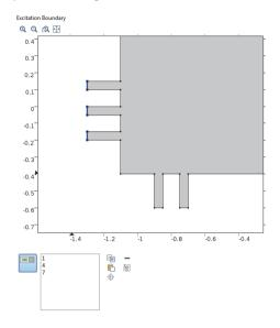
The user can here select boundaries by clicking directly in the graphics window, corresponding to the **Graphics** object, or by adding geometric entity numbers in a list of boundary numbers corresponding to a **Selection Input** object.
