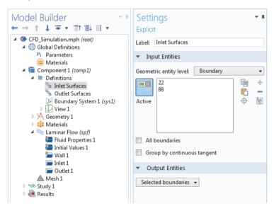
The figure below shows the **Settings** window for an **Inlet** boundary condition where the **Inlet Surfaces** selection is used. In this example, there is also an Outlet Surfaces selection.
