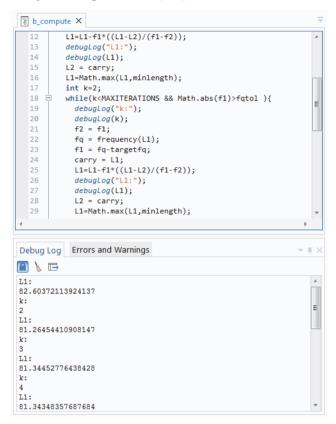
Use the debugLog command to display the value of variables in the **Debug Log** window. The code below illustrates using the debugLog command to display the values of strings and components of a 1D double array.
