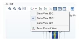
In addition to a list of all views, there is an option **Reset Current View** that will reset the currently active view to the state it had when the application was launched.
