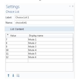
The vibrational modes 1–6 correspond to trivial rigid body modes and are not of interest in this application, hence the **Value** column starts at 7. The choice list allows you to hide the actual mode values in the model from the user by only displaying the strings in the **Display name** column. The first nonrigid body modes are named Mode 1, Mode 2, etc.
