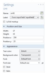
When adding an input field using the New Form wizard, a unit object is automatically added when applicable. By default, the unit is displayed using Unicode rendering. As an alternative, you can use LaTeX rendering by selecting the **LaTeX markup** check box. Then, the display of units will not depend upon the selected font.
