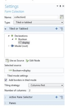
The tabbed mode is identical to a form collection with the **Type** set to **Tabs**. In tiled mode, all the forms are shown simultaneously in a grid. The layout for the tiled mode can be controlled by the settings in the subsection **Tiled mode settings**.
