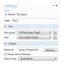
The **Filename** in its **Output** section is set to temp:///lineplot.txt.
