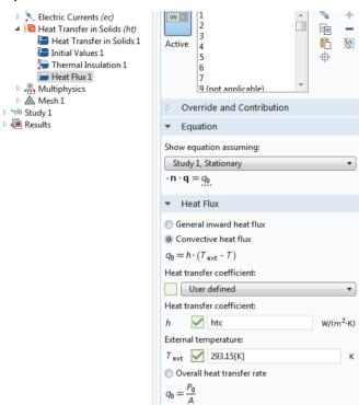
If you switch to the **Editor Tools** window, you will see additional nodes appear under the **Heat Flux** node. Right-click and use **Get** or **Set** to generate code in an active method window, as shown in the figure below.
