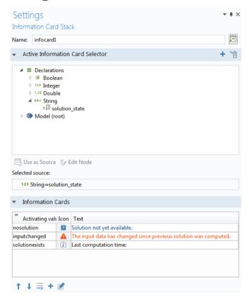
There are similarities with a **Card Stack** object, but for the **Information Cards**, each card has an icon and text. In the figure above, the string variable values nosolution, inputchanged, and solutionexists control which information card is shown.
