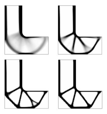
Figure 5: Topology optimization of the bracket, the material distribution, as defined by the finite element mesh, is modified to minimize the weight while satisfying a constraint on peak displacement. The design evolution is shown after 8, 16, 32 and 100 iterations.
