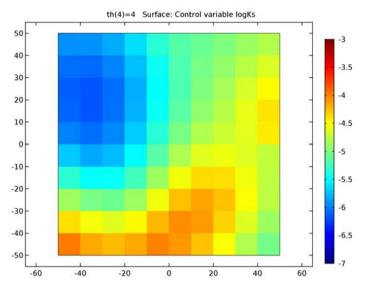
Figure 1: Hydraulic conductivity obtained by inverse modeling in the Aquifer Characterization model.
