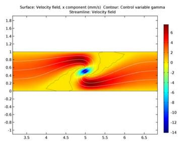
Figure 2: The horizontal velocity (surface plot) and velocity field (streamlines) after optimization. In addition, the contour  $\gamma = 0.5$  indicates the border between open channel and filling material.
